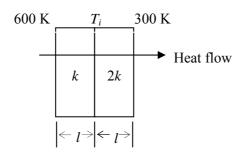
The interface temperature  $T_i$  (in K) of the composite wall is \_\_\_\_\_
